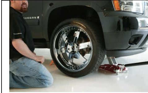
Raise and support front of vehicle frame on jack stands
