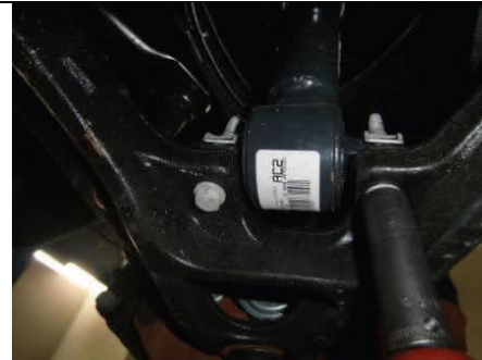
Remove lower strut mounting bolts
