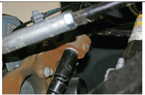
Tighten upper ball joint to spec.
