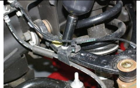
Disconnect ABS/brake bracket from upper control arm.
